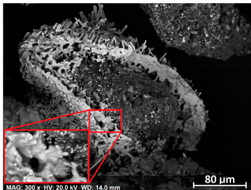
Figure 7. Fractured surface of a ferrochrome particle produced from chromite reduction by 180–300 \mu\text{m} charcoal, revealing the residual charcoal core with the presence of alloy nucleation on the core surface.
