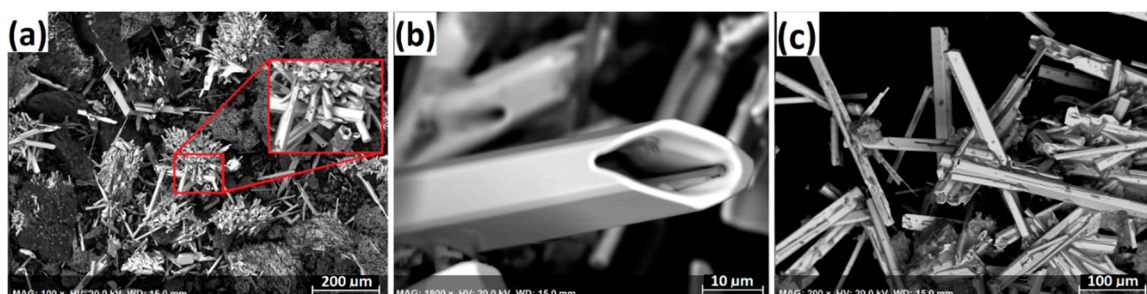
Figure 20. (a) Formation of ferrochrome mostly as M_7C_3 carbide whiskers in the reduced product from the large-scale segregation reduction of 37–75 \mu m chromite; in which (b) hollow hexagonal carbide whiskers were formed; and (c) ferrochrome carbide whiskers averaging about 200 \mu m in length have grown on the inner wall of the crucible during reduction.
